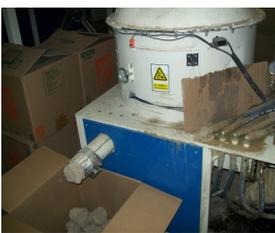
Paper fiber recovery from a machine connected to the plant’s air filtration system (new plant).
