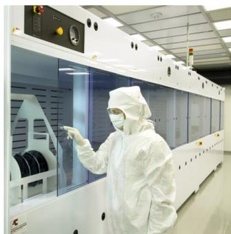
Silfex employee cleaning silicon parts operating a "wet bench". The employee wears clean room garments to prevent contamination of the work area and product once it has been cleaned.
